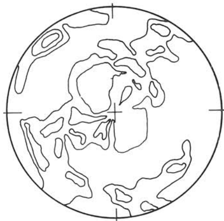
Fig. 5b. Sample B 4 (Bleicherode), detector slit 90 mm, counter level: 1.0; 1.5; 2.0; invest. No.: 584191152, (200) pole figure, NaCl.
